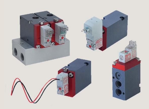
Clippard's EGV Series valves are an electronically piloted version of the GV series valves, ideal for large flow, low leak applications. Available in G1/8 ported and manifold mount, they utilize Clippard 10 mm or 15 mm valves, and offer numerous voltage and connection options. These 2/2 and 3/2 valves provide 10 times more flow than Clippard's MAV series and 2.5 times more flow than the MJV series! An externally piloted option is available for controlling lower pressures or other media.
